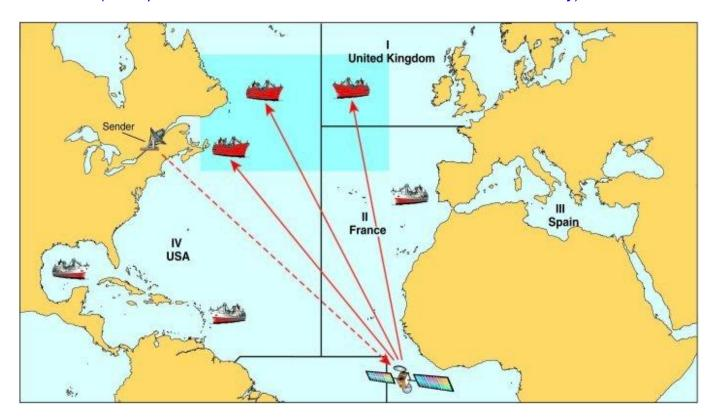
Figure 6 – SafetyNET message addresses to a rectangular area (All ships inside the addressed rectangle receive this MSI automatically)
