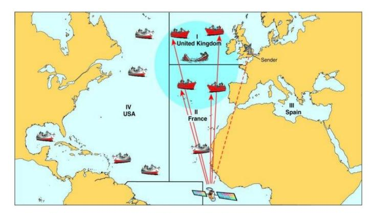
Figure 5 - SafetyNET message addressed to a circular area (All ships inside the addressed circle receive this MSI automatically)
